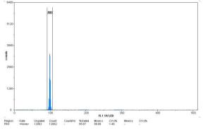
Calibration Beads UV 2.5  $\mu m$  measured on a CyFlow\* Space; Trigger = FL1
